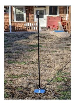
I used four 4" screws, a 3/8"-to-239 Stud, and a nice right angle adapter to make this work. I ended up making two sets of radials to test it out.
