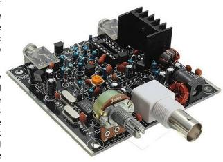
There were two toroids to wind, and neither was very hard, though the recommended lengths of magnet wire were far too short. I added an extra few inches (there was plenty of wire in the kit) and I'm glad I did. Oddly, the insulation on the magnet wire was not the usual stuff you can burn off with a bead of solder. I had to scrape it off with an X-acto knife and sandpaper.
