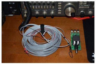
To pack it for travel, I coiled up the radiators and fastened them with strips of Velcro, then coiled up the feedline and secured that with a Velcro strap also. Total weight is 6.5 oz. To deploy it, I fastened the center snap to a 20 foot crappie pole and attached lengths of bank line to the ends of the radiators and stretched them out in an inverted V. You could also use slick line thrown over a tree branch instead of the fishing pole.
