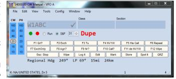
uppercase). Then click the "Section" textbox or hit Space and enter their section, "ct". At this point it's good to send your part of the exchange: "3A EMA". Finally, log the contact by clicking the "Log it" or hitting Enter.
